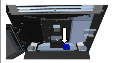
Vacuum the ash at the bottom of the pan and make sure the ash dump plug is in place and tight.
