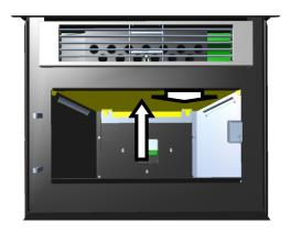
1. Lift the baffle and slide forward it a little to clear the supports.
