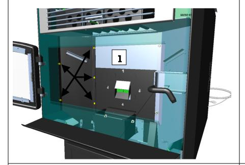
To access the exhaust ducts, remove the wall on the left side of the burning pot.
