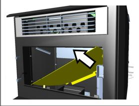
4. Continue rotating the baffle to remove it completely.
