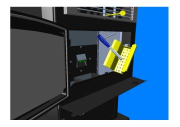
Using a scraper and a wire brush, thoroughly clean the surface of the burn pot. It is very important to leave no residue on the surface of the burn pot.
