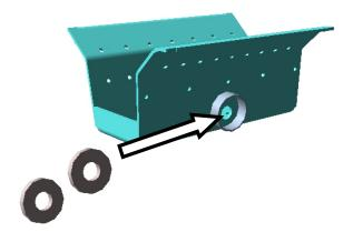
It is important to insert 2 Gaskets into the receptacle behind the burn pot.
