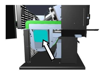
Remove the plate from the exhaust fan by unbolting the 4 bolts.
