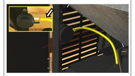
Remove the tube from the pressure sensor.
