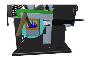
Vacuum the ash and clean the fins of the fan using a small brush.
